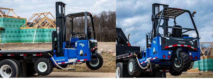
RGM+'s wireless remote control enables the operator to mount or dismount the forklift remotely while standing off either side of the road and away from traffic and the moving forklift. When using RGM+, operators benefit from the ability to enter or exit the forklift while the forklift is sitting flat on the ground. Finally, RGM+ provides the operator the ability to properly align the mounting hooks using the remote-operated side-shift function.
